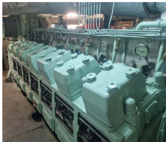
Figure 6. Engine fitted with analogue ex. temp. measuring devices (pyrometers)
