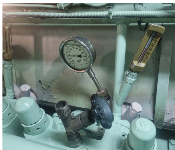
Figure 7. Indicator cock, pyrometer and cooling water thermometer
